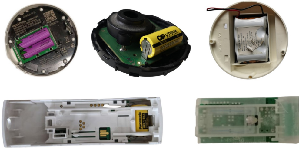
Figure 4: Different types of battery mounting in the considered electronic devices.
