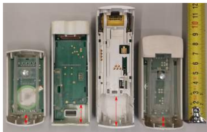
Fig. 2: Example electronic devices that need to be dismantled. Levering is used to remove the PCB from the housing.
