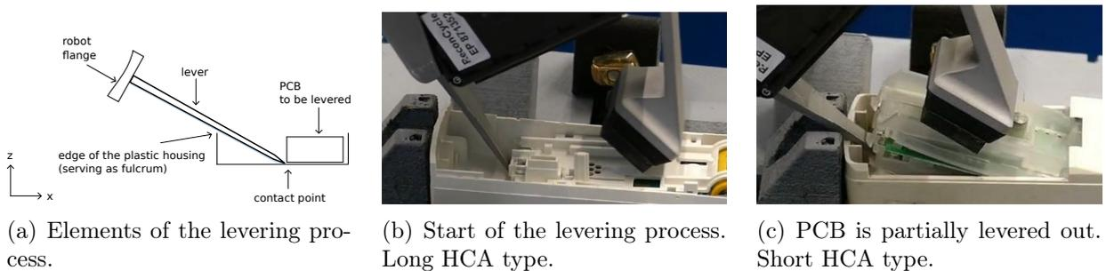
Figure 3: Adaptive levering
