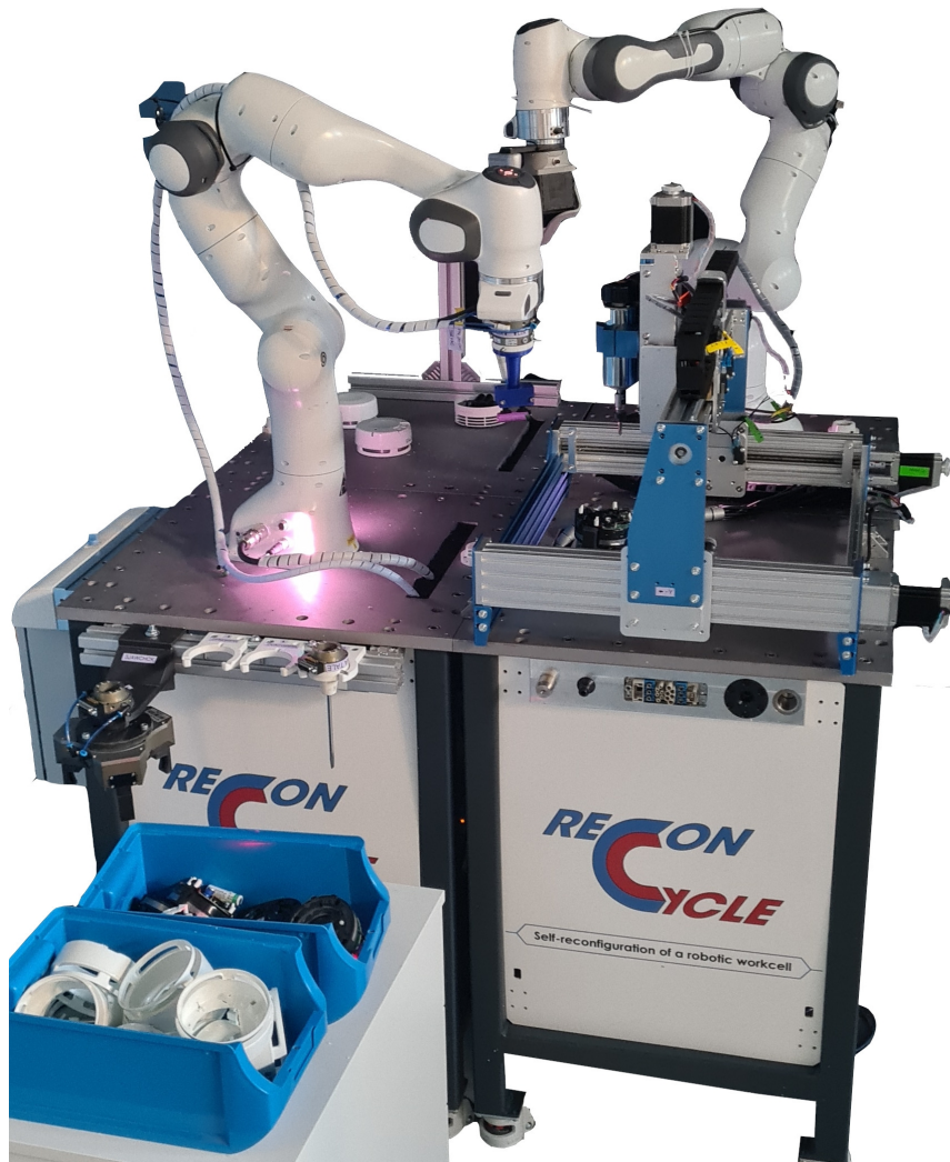
Figure 3: Workcell layout for smoke detector disassembly
