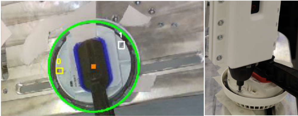
Figure 6: The image obtained by the camera including the screws detected and localized and the robot unscrew-driving the detected screw.
